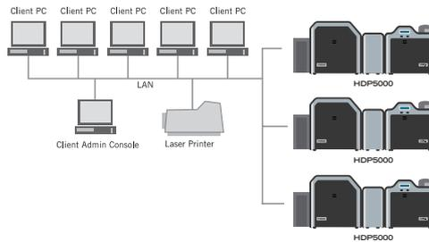
The HDP5000 can fit seamlessly into corporate IT infrastructures. Its onboard Ethernet port and print server provide the connectivity needed for networked operations.
